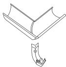
screws and silicon. For 45° corners cut gutter at 22.5°. \*For external corners in 150, allow extra 15mm on mitre cut to slip inside the opposite mitre cut for riveting and sealing.
